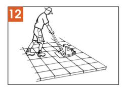
With a piece of carpet tied to the front of the compactor vibrate the pavers. This will lock in the gap sand & help to level any high spots. For small area's a thick piece of timber & a mallet will do the job.
