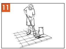
Always use kiln dried sharp gap sand. Ask for gap sand with additives that go hard as this will help prevent weeds & ants.
