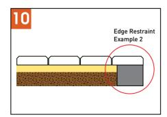
Edge restraint 2 - Create a cement beam approx 100mm in from the edge of the paver.
