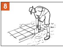
Using a space remove the excess road base & sand as you need to use and edge restraint on all the exposed edges. Note it's very important to restrain the paver, sand & road base.
