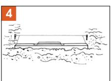
Using a screed, level an area to start from. For larger area's break them up into smaller & easier area's to mange.
