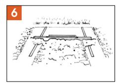
Lay the screed rail where just prepared. Place the screed on the rails & using a sawing motion pull the screed towards you. For larger area's simply repeat the process.
