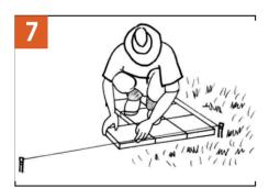
Set up a string line to suit the pattern you are going to lay & start laying.
