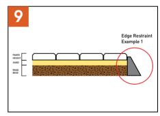
Edge restraint example 1 - Using the left over sand, mix with cement at a 4:1 ratio (4 shovels of sand to 1 shovel of cement).
